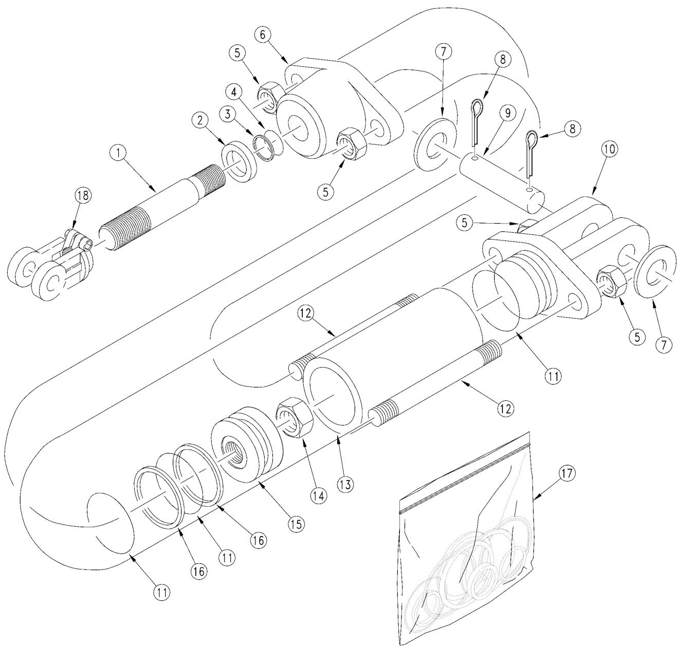
**Hydraulic Cylinder 1.5 x 2.5 x .75 Rod (810-555C)**
